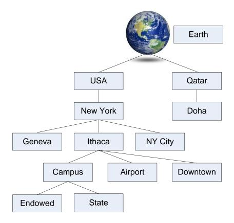
In the drawing, each of the blocks represents an "area," each of which may have named entities hierarchically beneath it. So most "facilities" on the Ithaca campus have a name in the EMCS that starts with the facility (usually building) name. But some EMCS points apply campus-wide or are considered part of the endowed or state campus infrastructure and having these "areas" in their names can be useful.
